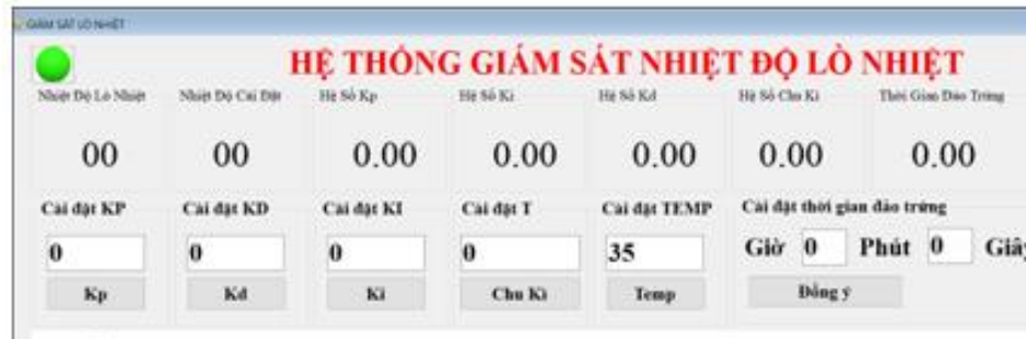
Figure 7: Software interface for monitoring and controlling egg incubator temperature
