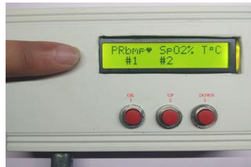
Figure 11: Placing finger on Max30100 sensor
