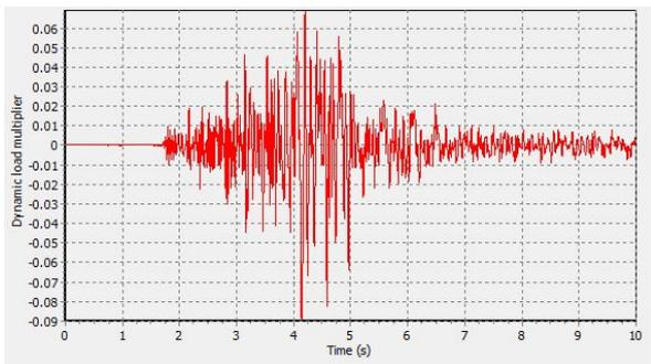
Figure 2: The trace of the 2001 Dien Bien earthquake.
