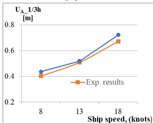
**Fig.9.** Relationship between significant amplitude of heave motion and ship speed in head wave.
