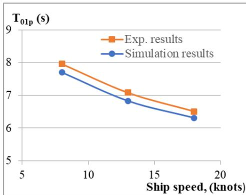
**Fig.7.** Relationship between average period of pitch motion and ship speed in head wave.
