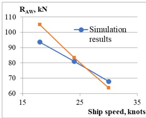
**Fig.6.** Relationship between added ship resistance and ship speed in head wave at  $h_s=2.41$  and  $T_p=9.775$
