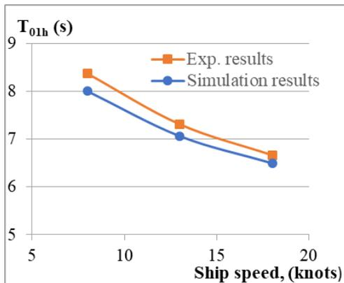
**Fig.8.** Relationship between average period of heave motion and ship speed in head wave.
