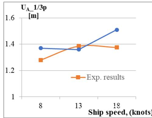
**Fig.10.** Relationship between significant amplitude of heave motion and ship speed in head wave.
