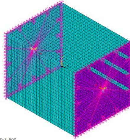
Figure 5. Boundary with coupling conditions.
