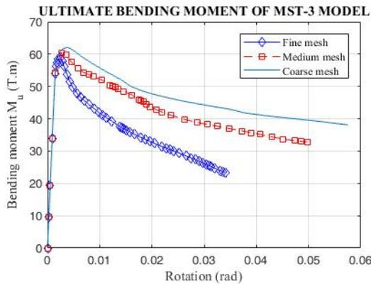
Figure 6. Bending moment of three mesh sizes.
