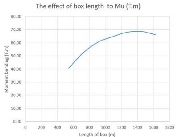
Figure 10. Bending moment of various length.
