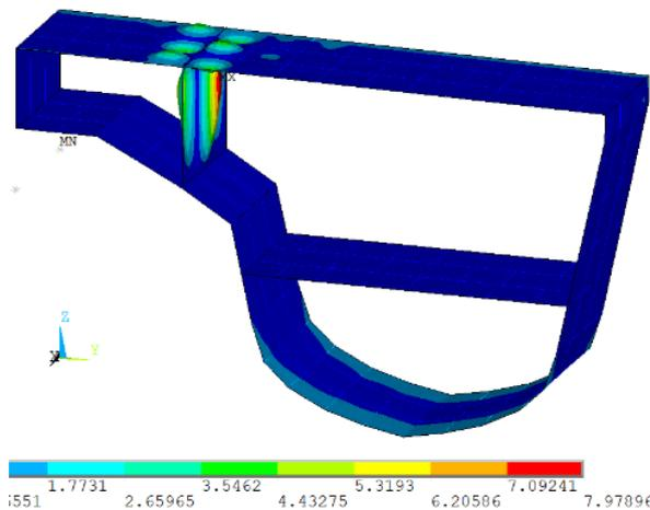
**Figure 16.** Deformation distribution without lateral pressure.
