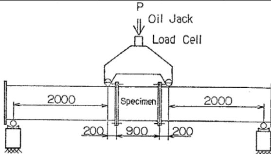
*Figure 1. Nishihara tested model setup.*
