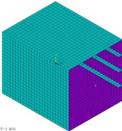
Figure 4. Medium mesh: Element size of  $b/5$ .
