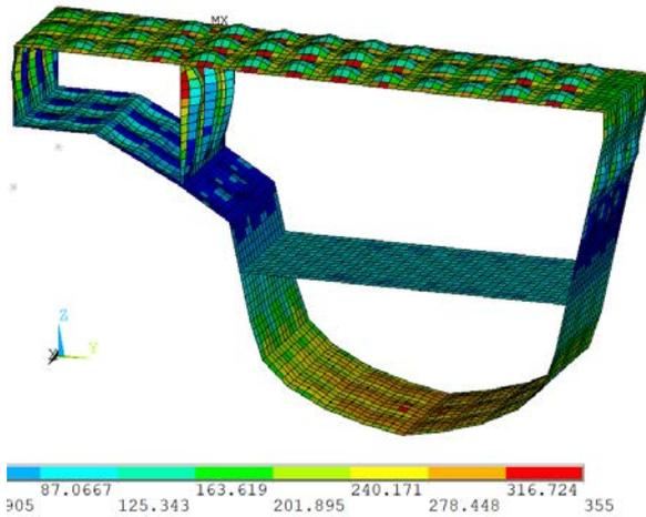
**Figure 15.** von-Mises stress distribution with lateral pressure.
