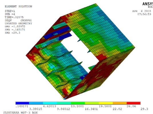
Figure 8. Von-Mises stress: medium mesh model.
