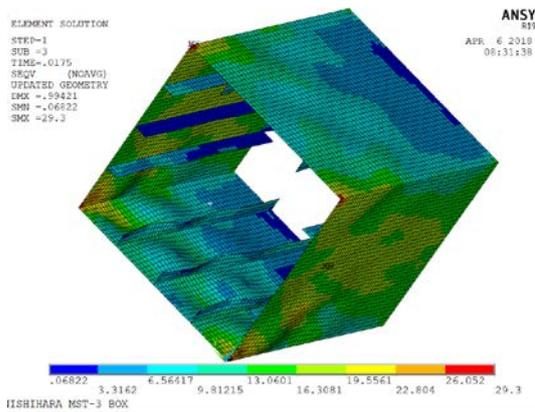
Figure 7. Von-Mises stress: fine mesh model.
