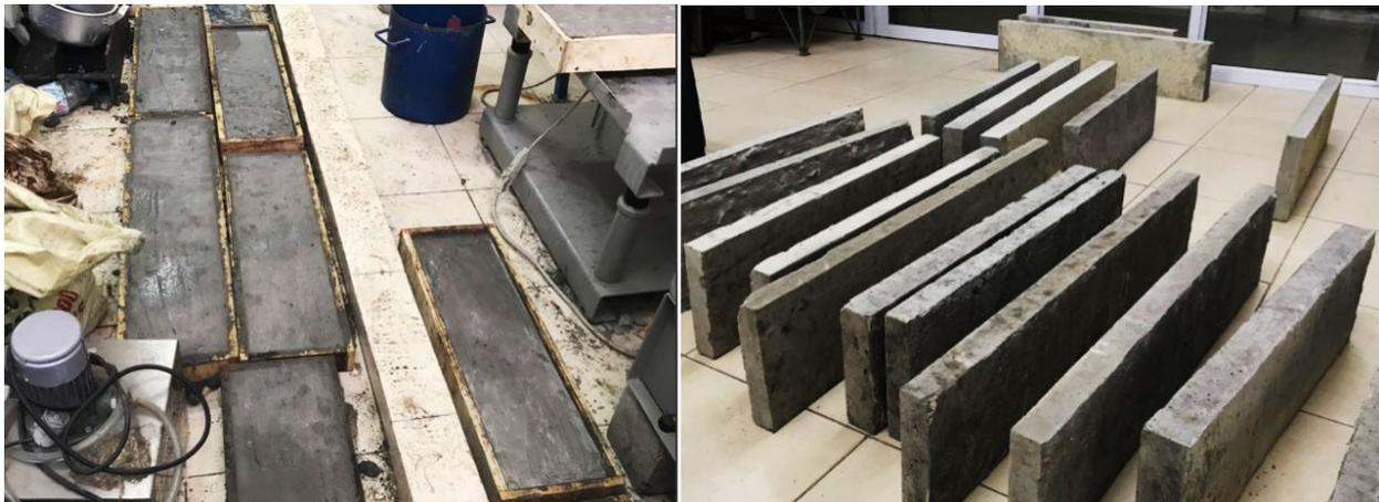
Figure 10. Concrete lagging.
