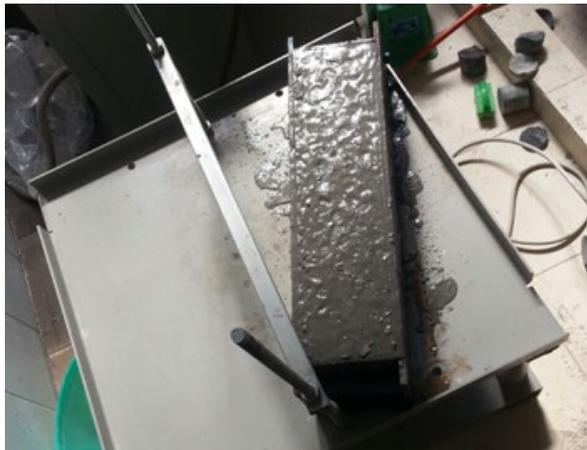
Figure 3. Specimen ready for tests on flexural strength values.
