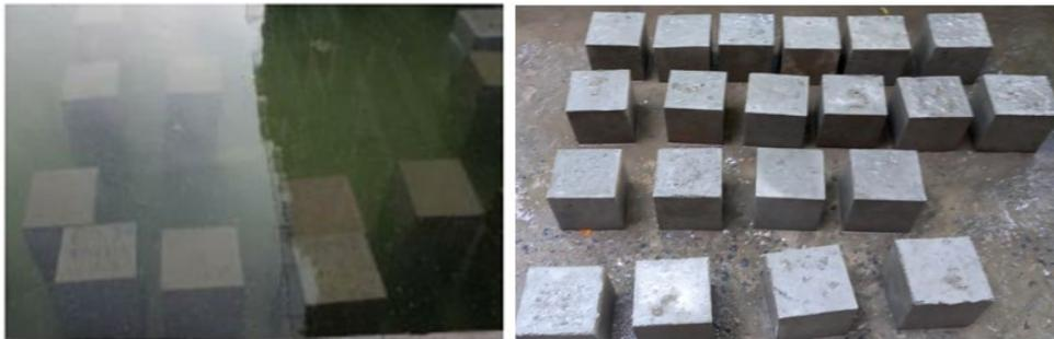
Figure 4. Curing of concrete cube.
