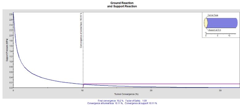
Figure 7. Safety factor in case of using the thickness of shotcrete 50 mm. (Received SF = 1.09).
