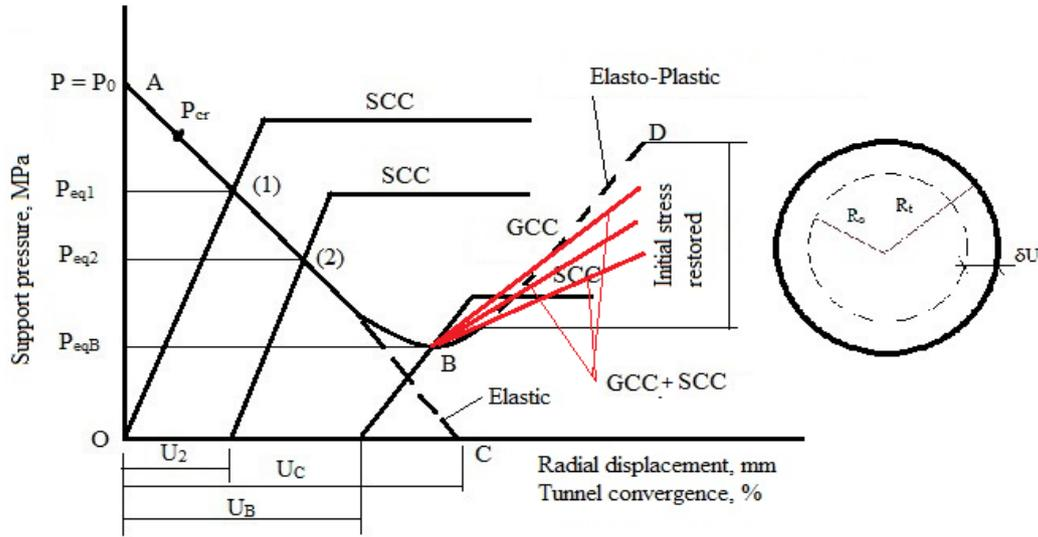
Figure 1. The Ground Characteristic Curve and Support.
