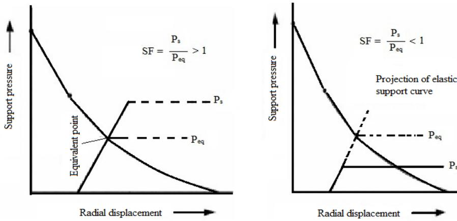
Figure 2. Defined the design of support according to Safety Factors (SF) (Carranza-Torres, 2004).
