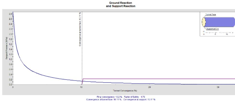
Figure 9. Final tunnel convergence and safety factor in case of shotcrete and rock bolts.
