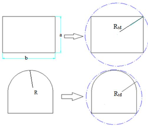
Figure 3. The conversion of rectangular and arch tunnels to analyze in Rocsupport 3.0.
