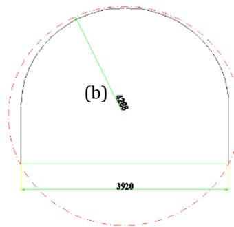
Figure 5. Equivalent cross-section to select rock support in drift: (a) Cross-section of drift; (b) Equivalent cross-section.
