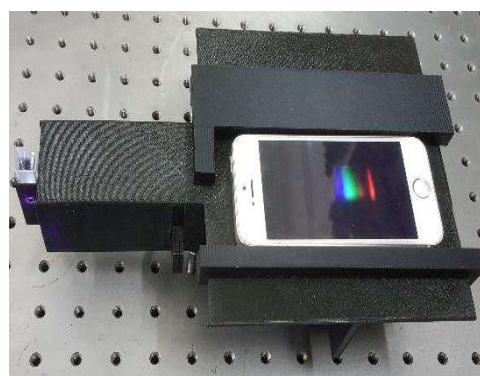
Figure 2. Final assembly of the smartphone-based sensor
