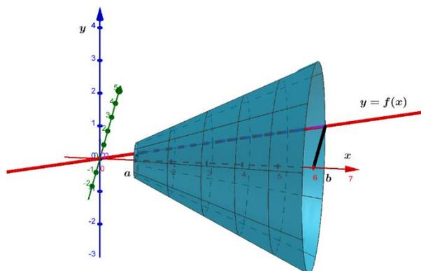
Figure 1. The graph  $y = f(x)$  - The plane region is bounded by the graph, the  $x$ -axis,  $x = a$  and  $x = b$  sweeps out a solid of revolution.
