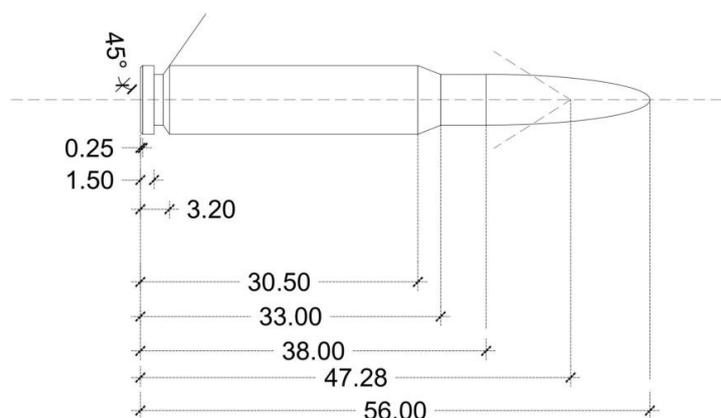
Figure 4: Dimensional parameters on the shell of the K56
