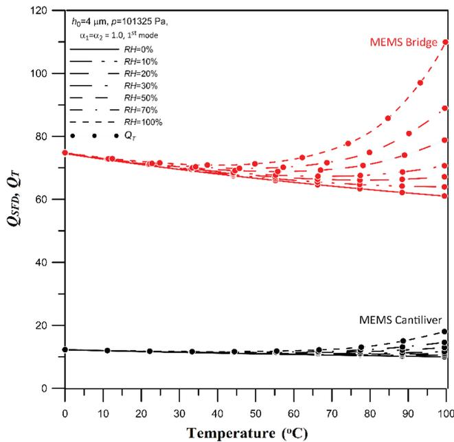
**Fig. 3. The quality factor by SFD ( $Q_{SFD}$ ) and total quality factor ( $Q_T$ ) versus ambient temperature ( $T$ ) for different relative humidity ( $RH$ ) values in the 1<sup>st</sup> modes of MEMS cantilever and bridge beam resonators at atmospheric pressure ( $p=101325$  Pa).**
