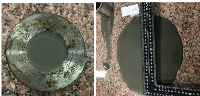
Fig. 3. Flow-slump of the tested binder.
