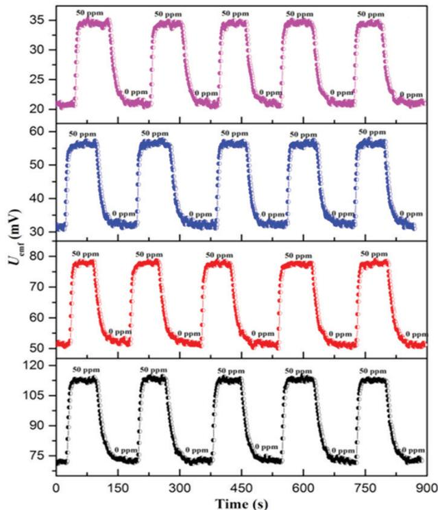
Fig. 5. Electromotive voltage ( $U_{emf}$ ) of the sensor Pt/YSZ/(Pt-WO<sub>3</sub>) responding to 50 ppm NO<sub>2</sub>/air cycles at operating temperatures of 450, 500, 550, and 600°C.
