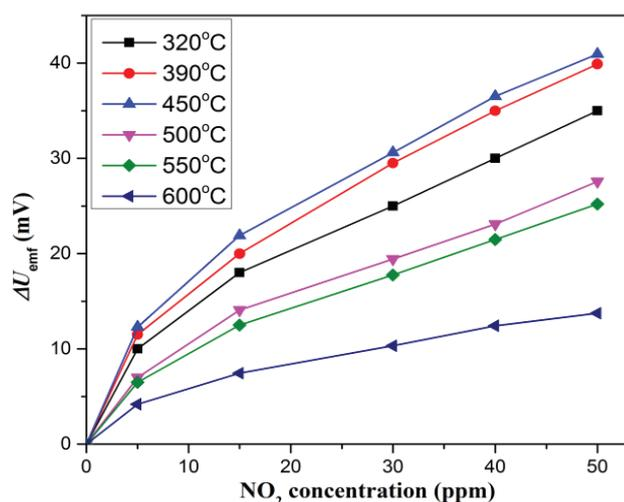
Fig. 6. Dependence of sensing response ( $\Delta U_{emf}$ ) of the Pt/YSZ/(Pt-WO<sub>3</sub>) sensor on NO<sub>2</sub> concentration at operating temperatures of 320, 390, 450, 500, 550, and 600°C.
