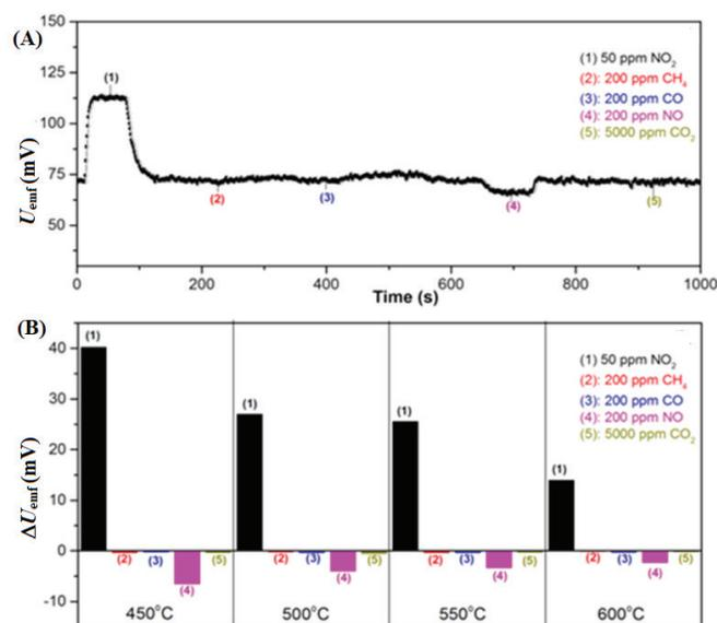
Fig. 7. (A) Typical electromotive voltage ( $U_{emf}$ ) of the Pt/YSZ/(Pt-WO<sub>3</sub>) sensor responding to 50 ppm NO<sub>2</sub>, 200 ppm CH<sub>4</sub>, 200 ppm CO, 200 ppm NO, and 5000 ppm CO<sub>2</sub> at 450°C and (B) Comparison of the sensing response ( $\Delta U_{emf}$ ) for these gas concentrations at operating temperatures of 450, 500, 550, and 600°C.
