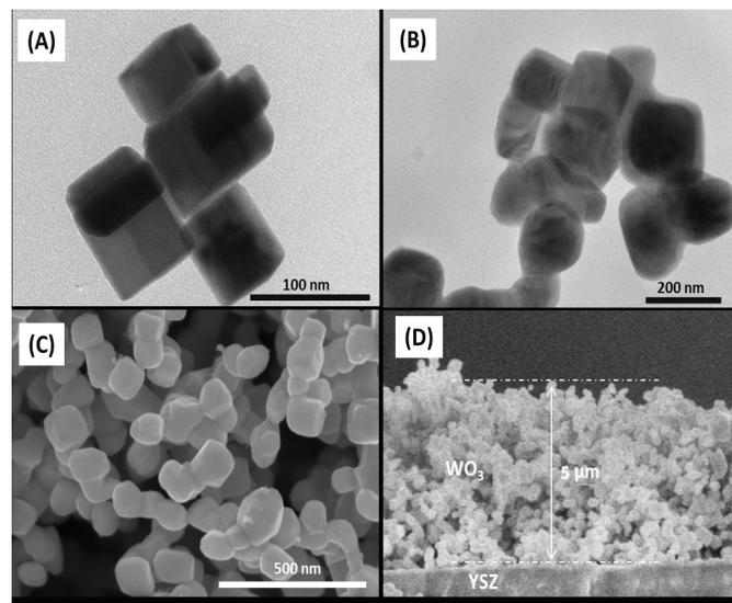
Fig. 2. (A) TEM images of as-synthesised  $\text{WO}_3$  nanoparticles, (B)  $\text{WO}_3$  nanoparticles originated from the sensing electrode after sintering at  $700^\circ\text{C}$ , (C) SEM images of surface, and (D) Cross-sectional view of the  $\text{WO}_3$  sensing electrode on YSZ substrate.
