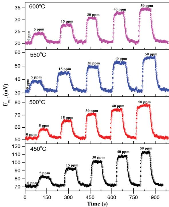
Fig. 4. Electromotive voltage ( $U_{emf}$ ) of the sensor Pt/YSZ/(Pt-WO<sub>3</sub>) responding to 5, 15, 30, 40, and 50 ppm NO<sub>2</sub> at operating temperatures of 450, 500, 550, and 600°C.
