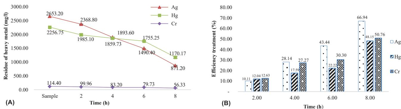
Fig. 7. Effect of electrolysis time on (A) heavy metal concentration and (B) efficiency of removal of heavy metals from COD wastewater.
