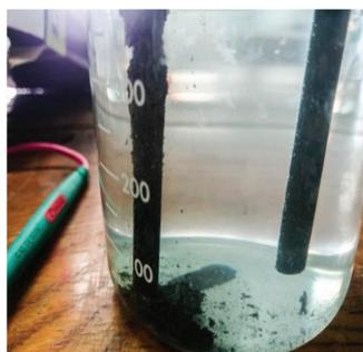
Fig. 4. Electrolyte product falling off the electrode.
