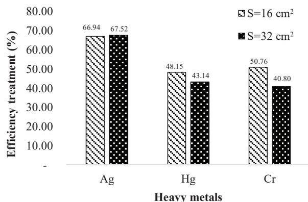
Fig. 10. Comparison of the treatment efficiency of heavy metals between the two electrode areas, 16 and 32 cm<sup>2</sup>, for t=8 h.
