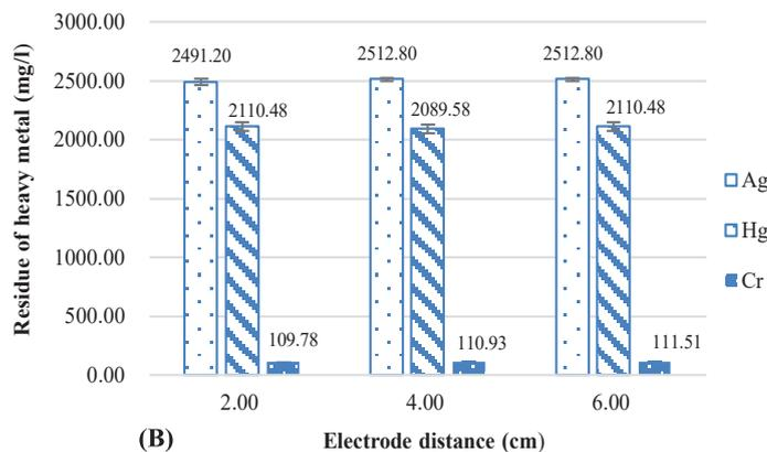
Fig. 6. Effect of the distance between electrodes on (A) the current, (B) the effect of heavy metal removal in COD wastewater treatment.
