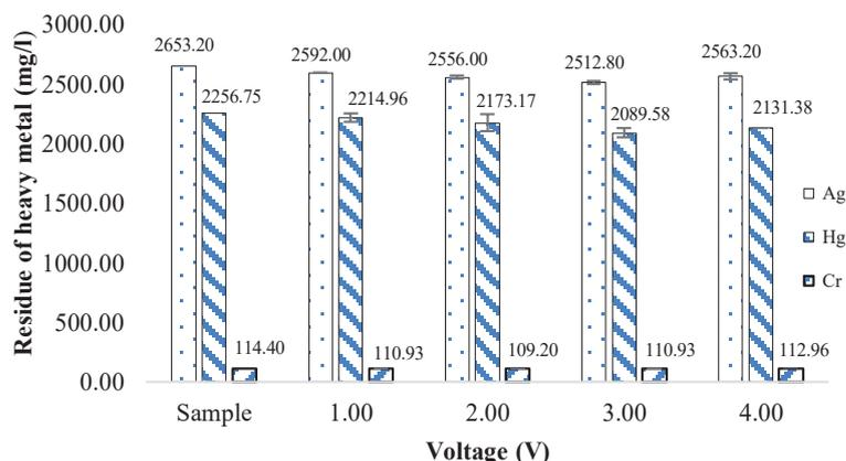
**Fig. 3. Effect of voltage on removal of heavy metals.**
