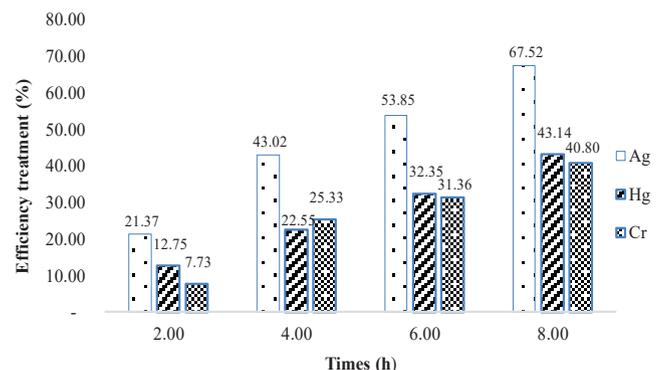
Fig. 9. The removal efficiency of heavy metals over electrolysis time.
