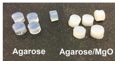
Fig. 1. Photograph of agarose and cylindrical agarose/MgO units.
