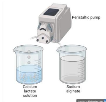
Figure 2. Ca-alginate gel beads formation.
