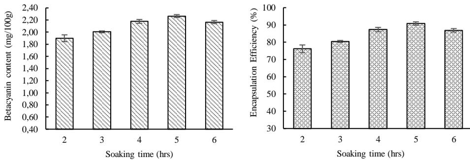
Figure 6. Effect of soaking time on the betacyanins content in bead and encapsulation efficiency
