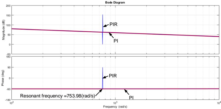
Figure 3. Bode diagram of open-loop PI and PIR controllers.
