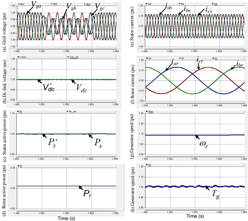
Figure 9. Performance of DFIG wind turbine system for unbalanced voltage sag (in pu).
