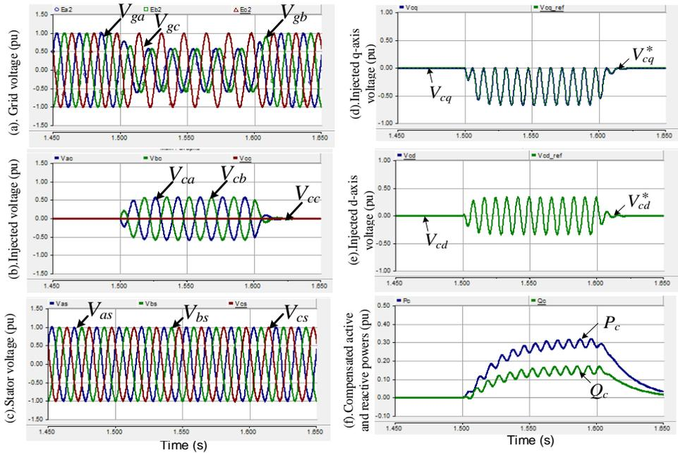
Figure 8. Performance of series grid-side converter system for unbalanced voltage sag (in pu)
