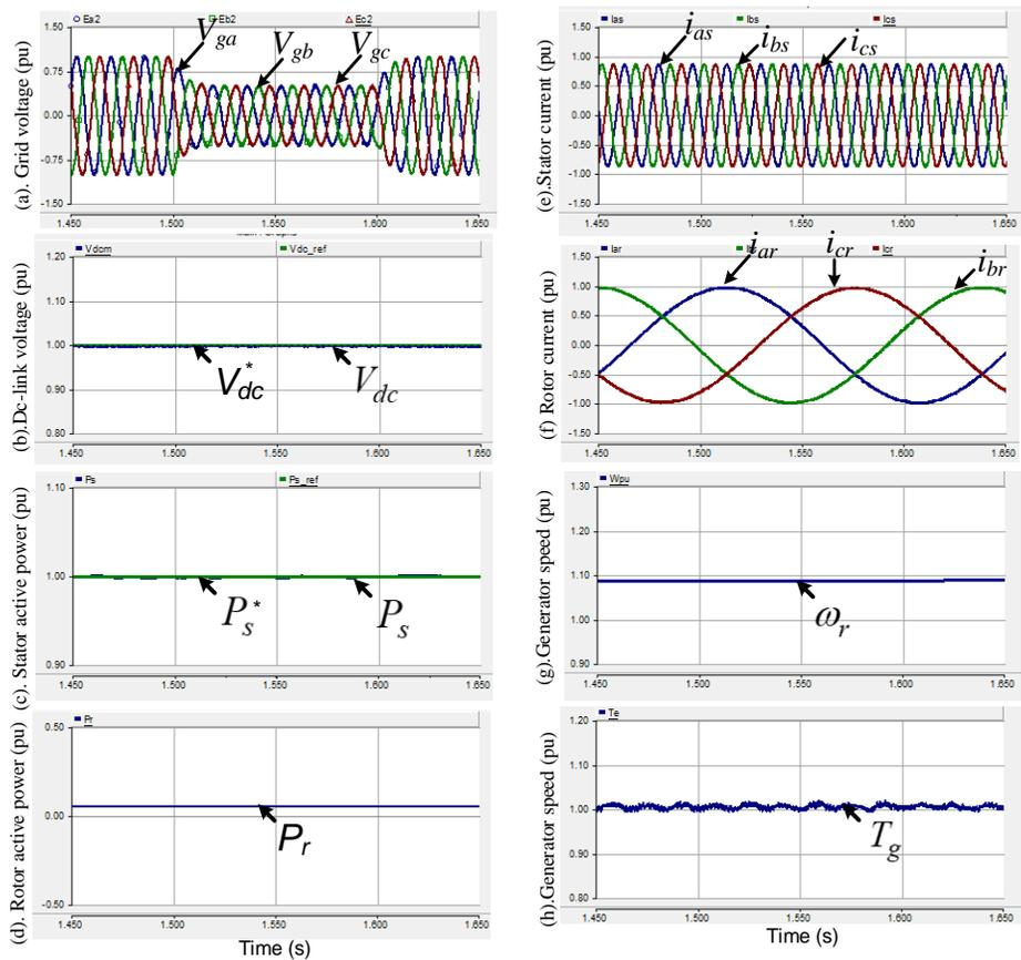
Figure 6. Performance of DFIG wind turbine system for balanced voltage sag (in pu).
