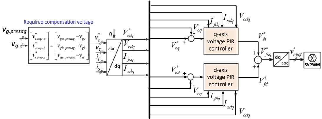
Figure 2. Voltage control block diagram of SEGSC.
