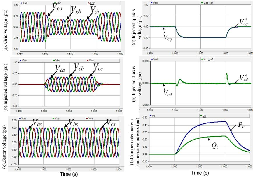
Figure 5. Performance of series grid-side converter system for balanced voltage sag (in pu).
