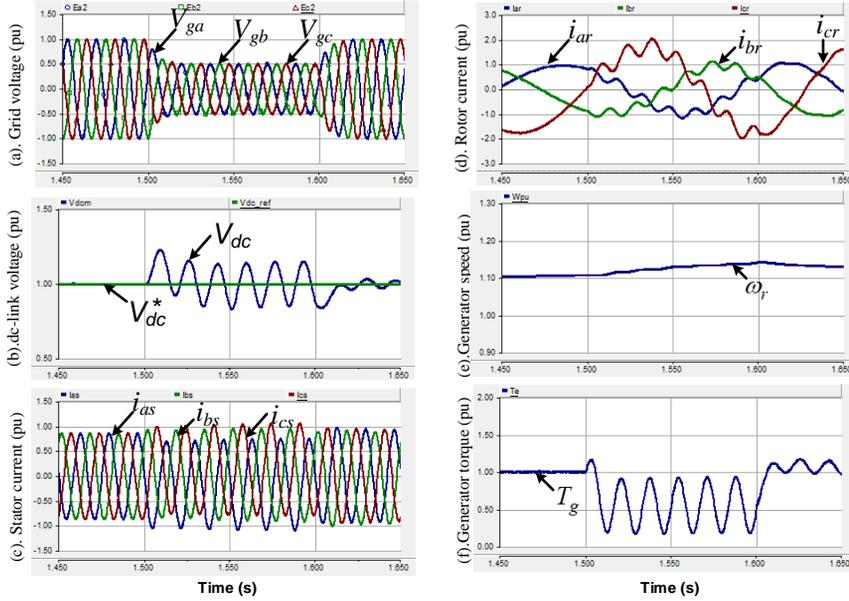
Figure 4. Performance of DFIG wind turbine system for balanced voltage sag (in pu).
