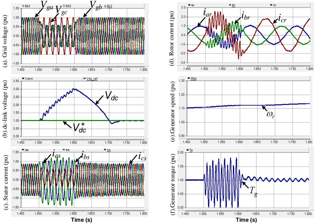
Figure 7. Performance of DFIG wind turbine system for unbalanced voltage sag (in pu)
