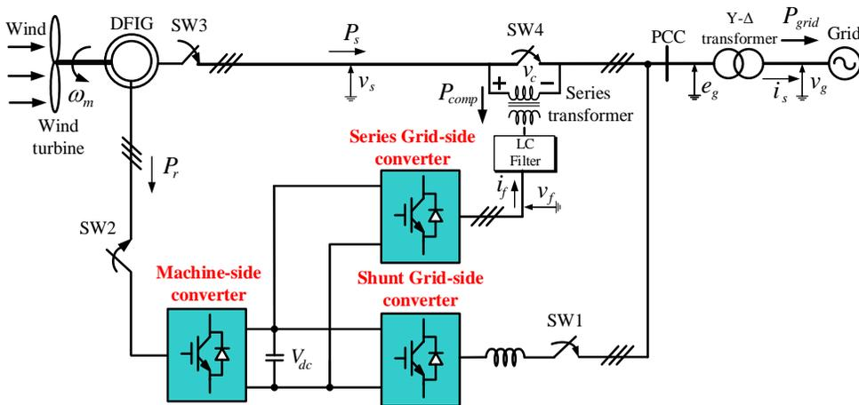
Figure 1. DFIG wind turbine system with SEGSC.
