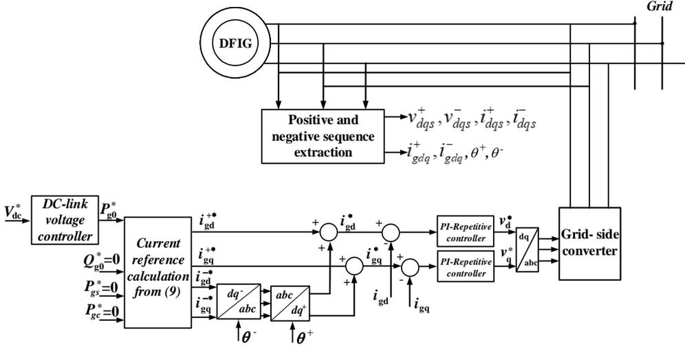
Figure 5. Control diagram of grid-side converter under unbalance grid voltage.
