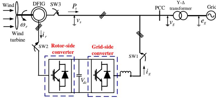
Figure 1. Circuit configuration of DFIG wind turbine system
