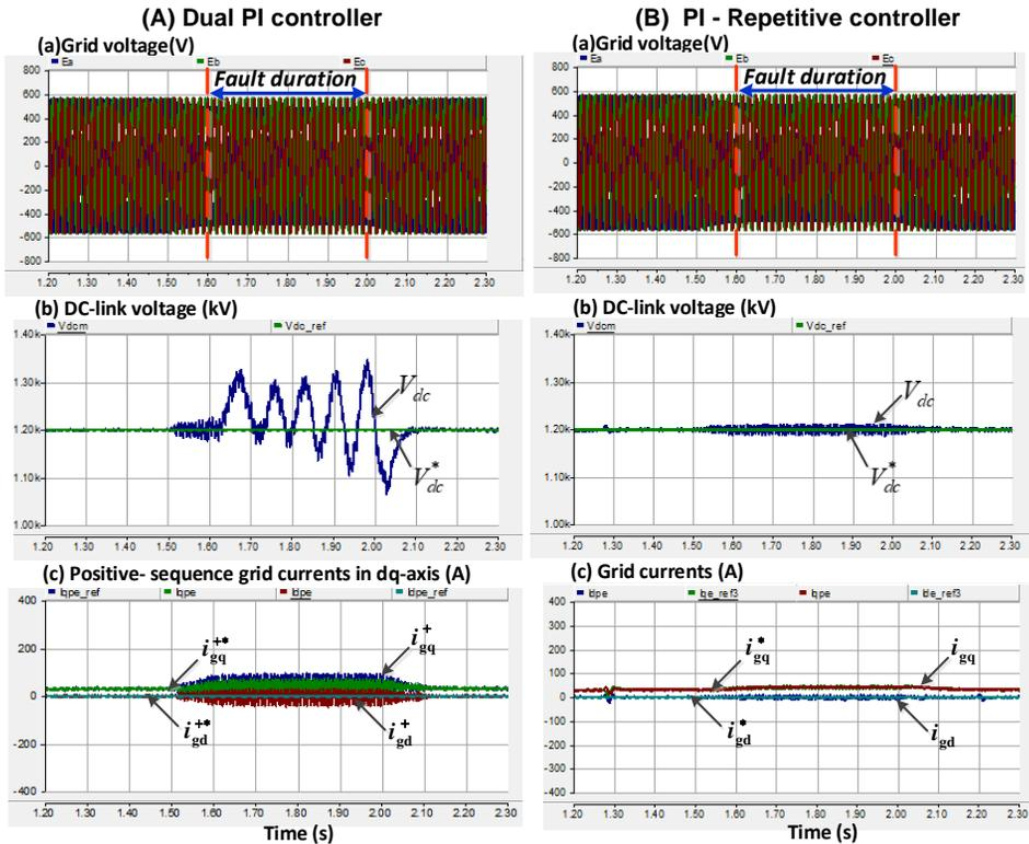
Figure 7. Control performance of grid-side converter for grid phase-A voltage sag (14%) in 2 cases: (A) Dual PI control [6]. (B) Proposed method. (a) Grid voltage. (b) DC-link voltage. (c) Grid current.
