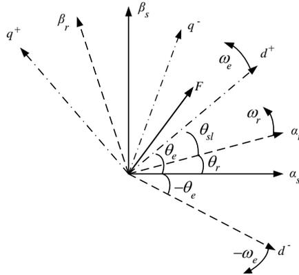
Figure 2. Relation between the  $\alpha_s \beta_s$ ,  $\alpha_r \beta_r$  and  $dq^+$ ,  $dq^-$  reference frames.
