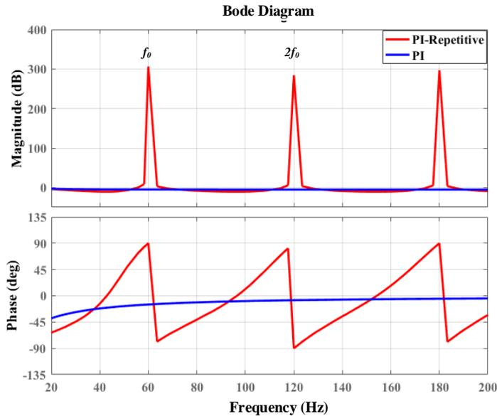
Figure 4. Bode plots for the PI and PI-Repetitive controllers.
