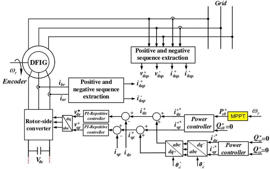
Figure 3. Control diagram of rotor-side converter under unbalance grid voltage.
