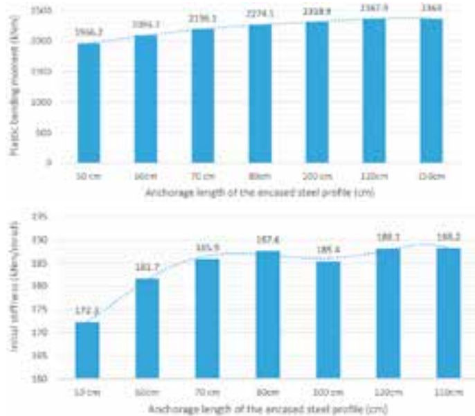
Figure 9. Plastic bending moment and initial stiffness in cases of different anchorage length
