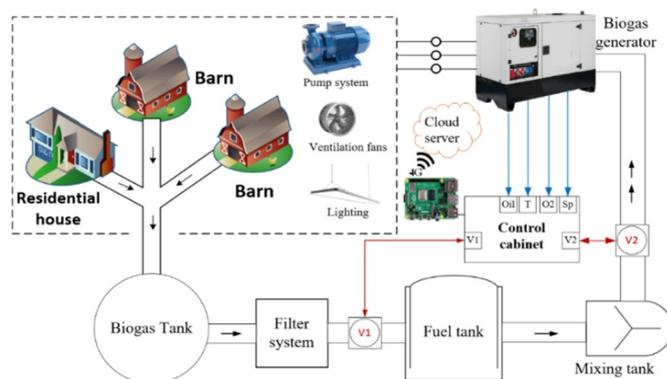
Figure 1. The livestock farm equipped with biogas-based generation systems and typical electrical loads.
