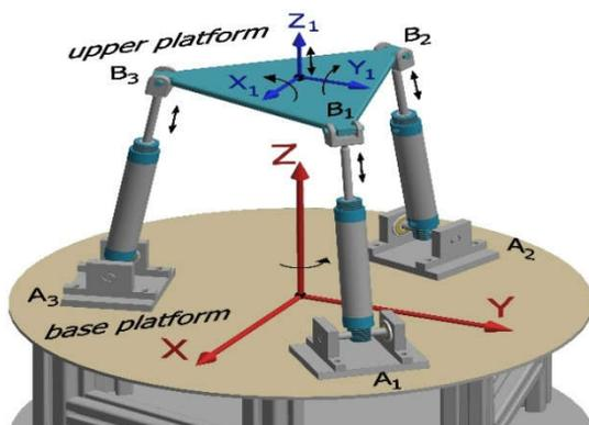
Figure 1. 4DOF car driving simulator system
