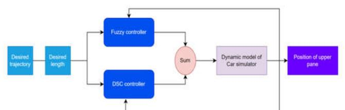
Figure 3. Block diagram
