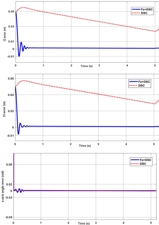
Figure 6. Tracking errors of  $l_1$ ,  $l_2$ ,  $l_3$  and  $\gamma$
