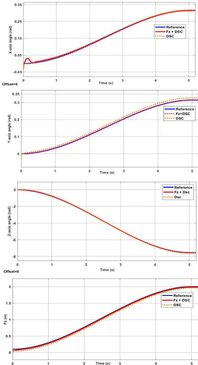
Figure 4. Trajectories of  $\alpha$ ,  $\beta$ ,  $\gamma$  and  $P_z$
