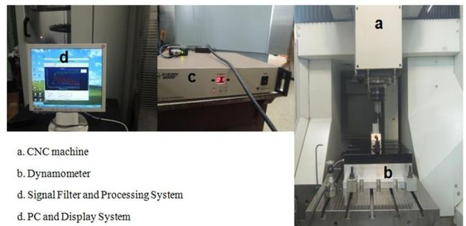
Fig. 15. Setup measurement of cutting force setting
