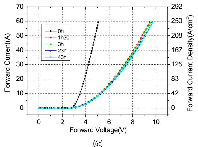
Figure 6. Forward characteristics evolutions of 2mm<sup>2</sup> (6a), 8mm<sup>2</sup> (6b) and 24mm<sup>2</sup> (6c) diode
