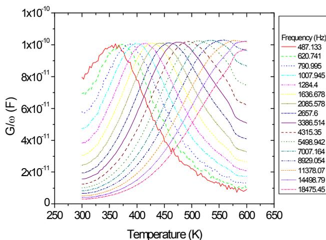
Figure 7. Normalized conductance vs. temperature for 16 different frequencies obtained on a stressed diode
