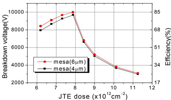
Figure 2. Diode blocking voltage and efficiency percentage evolution in function of active JTE dose for two different etching depths
