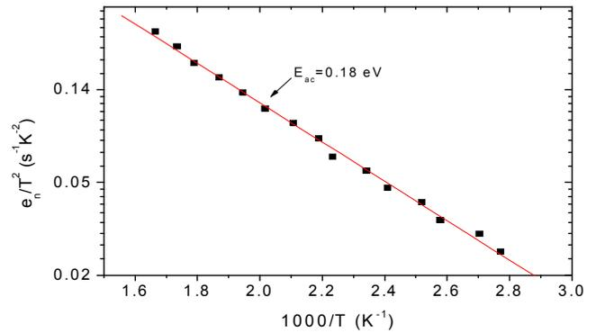
Figure 8. Arrhenius plot of the defect signature
