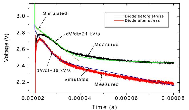
Figure 9. Measured and simulated curves OCVD voltage transient characteristics of a diode before and after electrical stress
