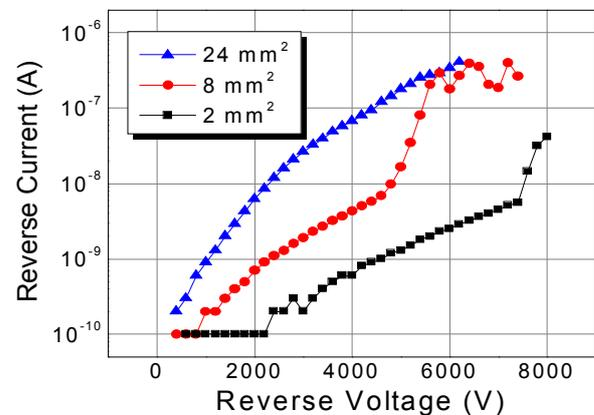
Figure 3. Reverse characteristics of the best fabricated 6.5kV diodes for three different areas
