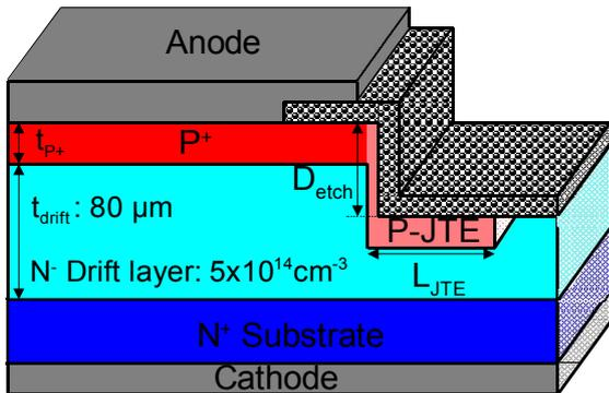
Figure 1. Schematic cross-section of the 6.5kV 4H-SiC bipolar diodes
