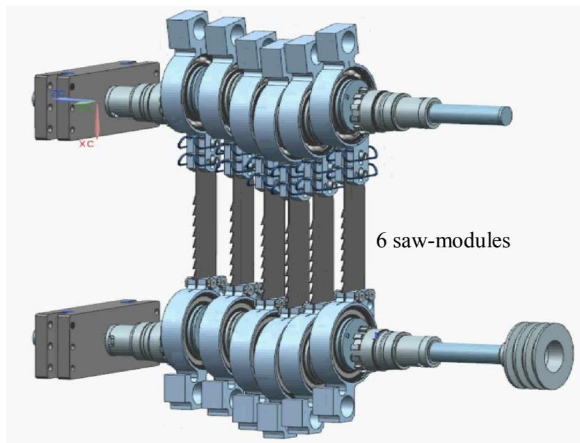
**Fig. 1.** An innovative frame saw machine with 6 saw-modules
