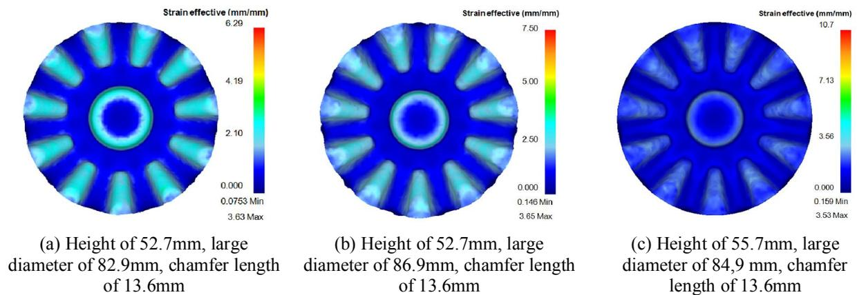
Fig. 6. An representative output of simulation
