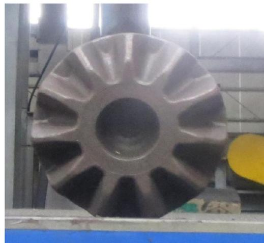
Fig. 11. Forged bevel gear
