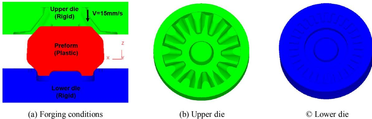
Fig. 5. Simulation model of the forming stage
