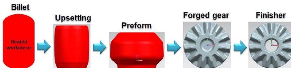
Fig. 1. Bevel gear forging process
