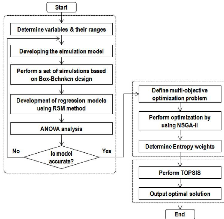
**Fig. 4.** Systematic procedure for the simulation-based design of experiments and optimization
