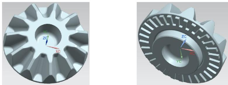
Fig. 2. Forged bevel gear
