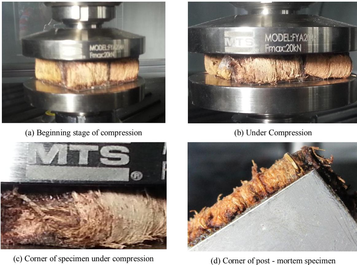
**Figure 7.** photographs showing deformation of mesocarp sandwich panel
