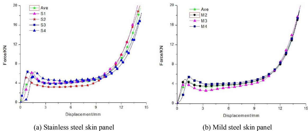
**Figure 6.** The Force -displacement curves of the mesocarp core sandwich panels under quasi-static compression
