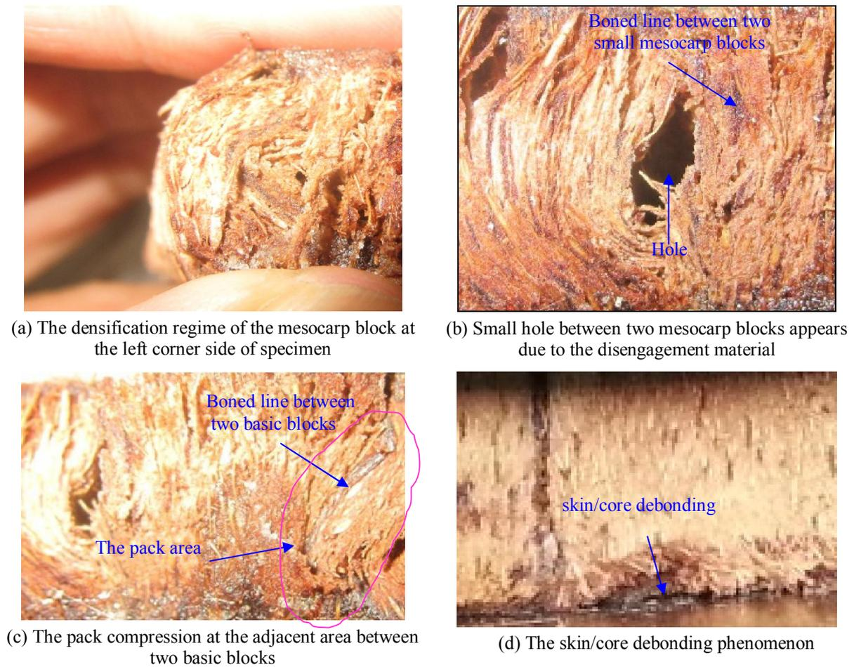
**Figure 8.** Photographs showing the deformation and failure of the mesocarp sheet core during the test.
