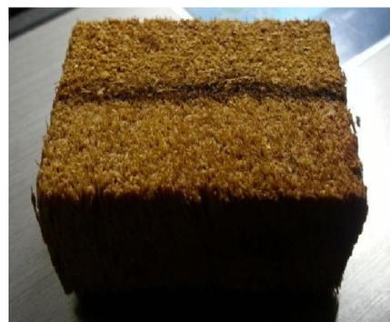
(b) Gluing two mesocarp blocks together
