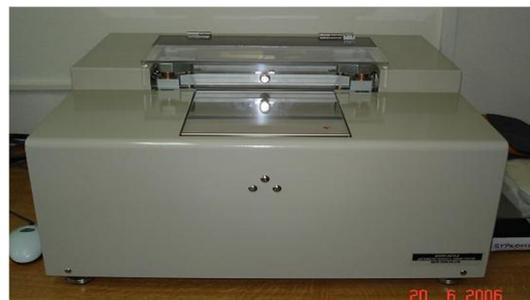
Fig. 1. KES-FB1 device to determine the tensile properties of the fabric
