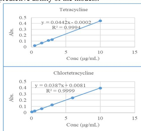
Figure 3. The plots of Beer – Lambert’s law of absorbance for (A) tetracycline at 269.20 nm and (B) chlortetracycline at 266.80 nm
