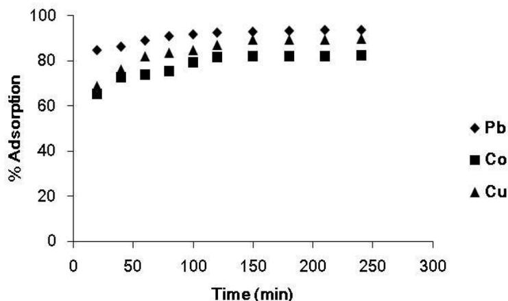
Fig. 4. Effect of contact time on adsorption of heavy metals by  $\gamma$ - $\text{MnO}_2$  nanostructure ( $\text{pH} = 4$ , agitation speed = 240 rpm, Mass = 0.1 g and Temp =  $24^\circ\text{C}$ )
