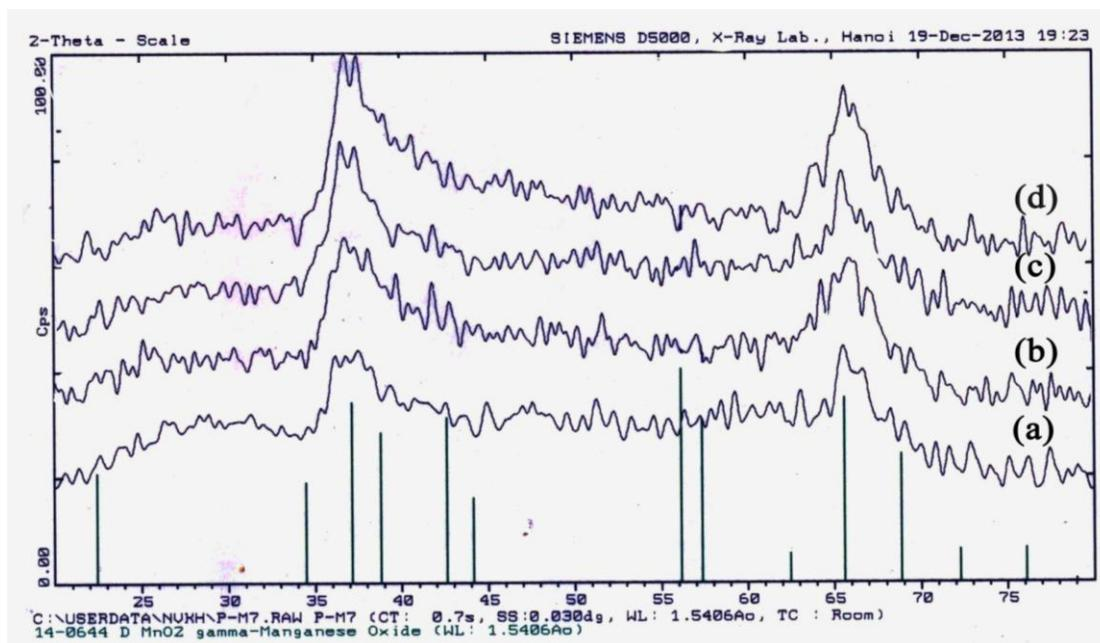
Fig. 1. XRD image of prepared sample ( $\gamma$ - $\text{MnO}_2$ ) at different shaking speed: (a) at 480 rpm, (b) at 600 rpm, (c) at 720 rpm, (d) at 840 rpm.
