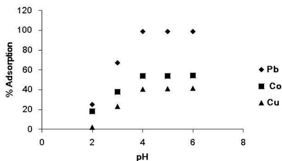
Fig. 3. Effect of pH on the adsorption of heavy metals by  $\gamma$ - $MnO_2$  nanostructure
