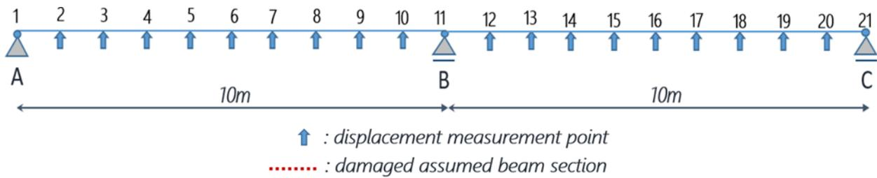
Figure 11: Illustration of two-span continuous reinforced concrete beam in SAP2000.
