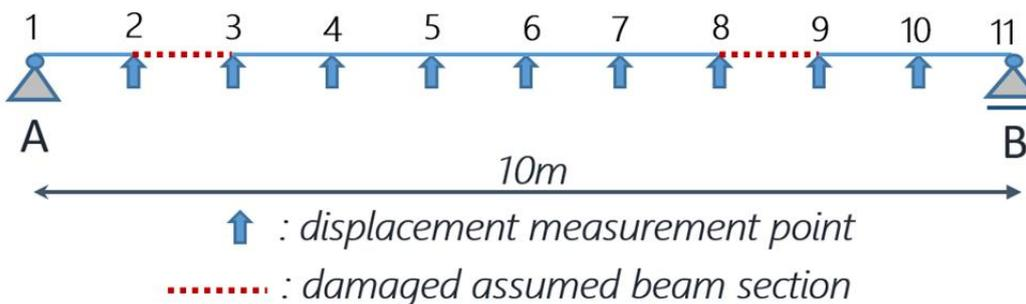
Figure 6: Simple beam diagram assuming two damages at the 2<sup>th</sup> and the 8<sup>th</sup> elements.
