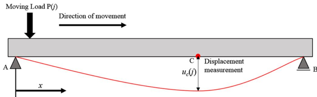
Figure 1: Illustration of the displacement influence line.
