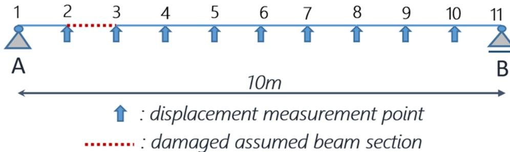
Figure 4: Simple beam diagram assuming damage at the second element.
