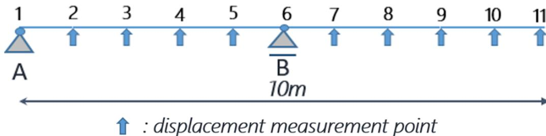
Figure 15: Illustration of overhanging beam in SAP2000.
