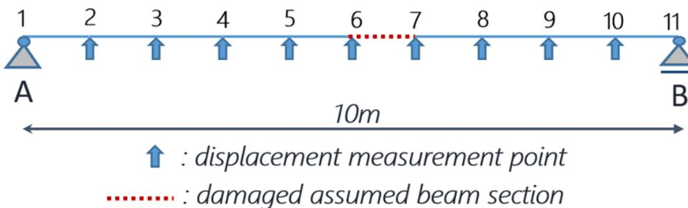
Figure 5: Simple beam diagram assuming damage at the 6<sup>th</sup> element.
