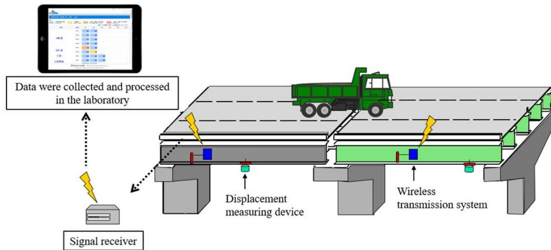
**Figure 18:** Proposing diagnostic procedures for bridges.
