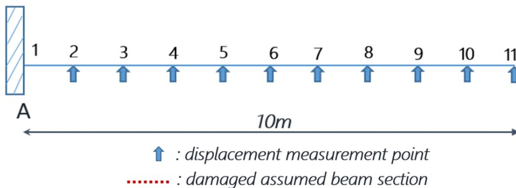
Figure 13: Illustration of cantilever beam in SAP2000.
