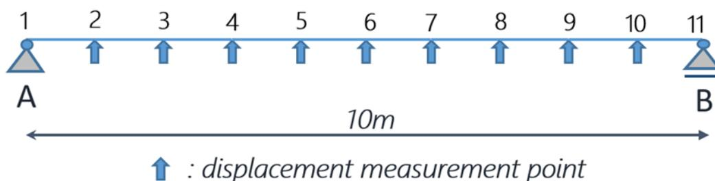
Figure 2: Illustration of single-span simple beam in SAP2000.
