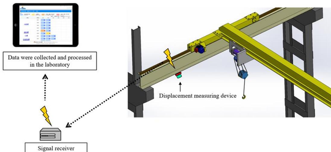
**Figure 17:** Proposing diagnostic procedures for crane girders.
