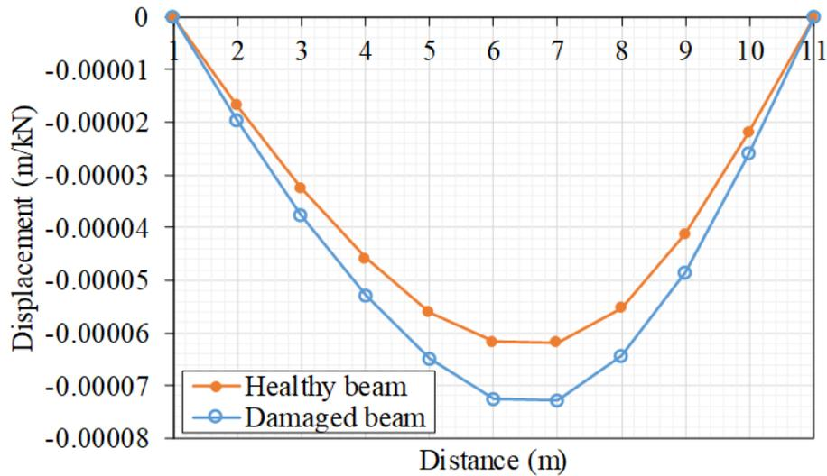
**Figure 7:** Influence line obtained at position 6 of healthy and damaged beams.
