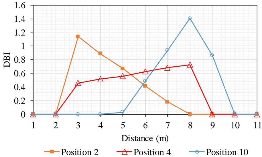
Figure 10: Diagnostic results of the damaged location of Case 3
