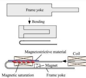
**Figure 2:** Frame (top) and device configuration (bottom)
