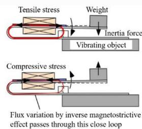
**Figure 3:** Principle of power generation: Inertial force downward (top) and upward (bottom)
