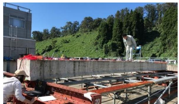
**Figure 6:** Impact test on the PC girder
