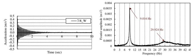
Figure 7: Vibration test result (Measuring point: 7L/8)
