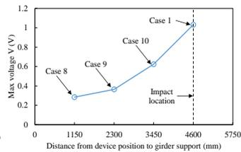
**Figure 12:** Effect of device location on generated voltage
