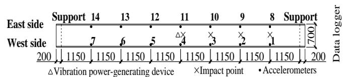
**Figure 5:** Sensor layout of cases 1, 5, 6, and 7
