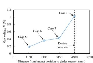
**Figure 11:** Effect of impact location on generated voltage
