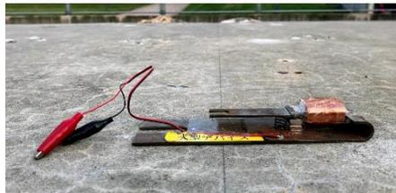
**Figure 1:** A prototype vibration power generator
