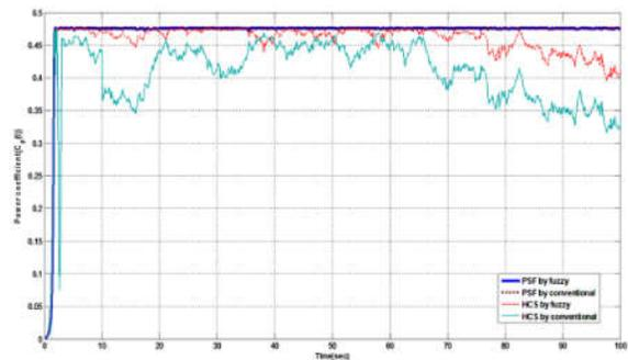
**Figure 11. Power coefficient profile**
