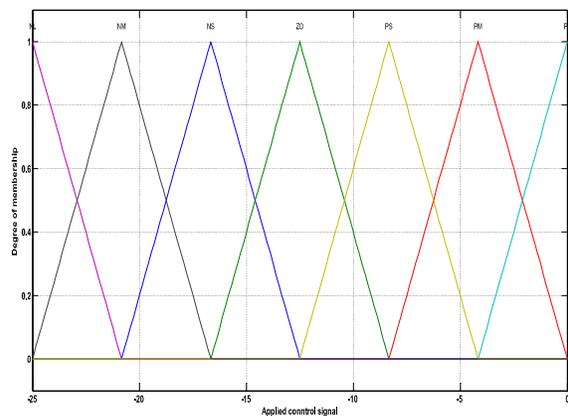
Figure 9. Membership function of control signal
