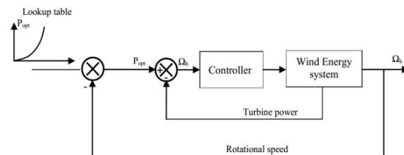
Figure 4. Block diagram of power signal feedback
