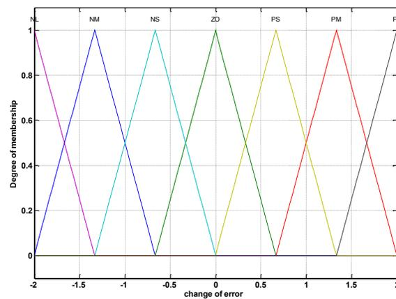
Figure 8. Membership function of change of error
