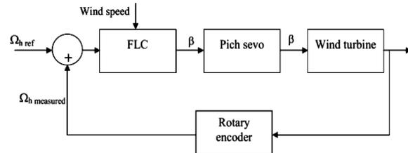
**Figure 5. A block diagram of pitch angle control of wind turbine using FLC**
