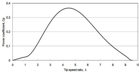
Figure 2. Power coefficient  $C_p$  versus tip speed ratio
