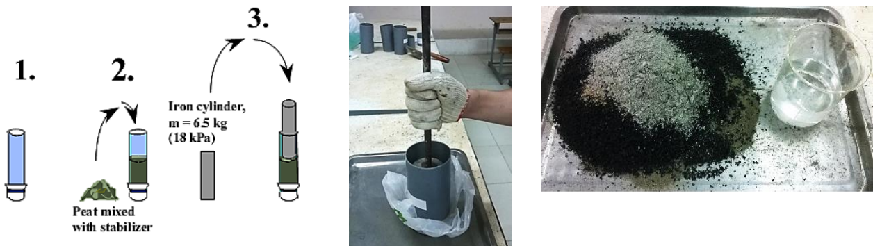
Figure 1. Material mixing. a) Procedure of soil compaction ; b) Mixture prepare
