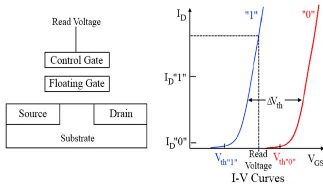
Fig. 2. Floating-gate reading operation
