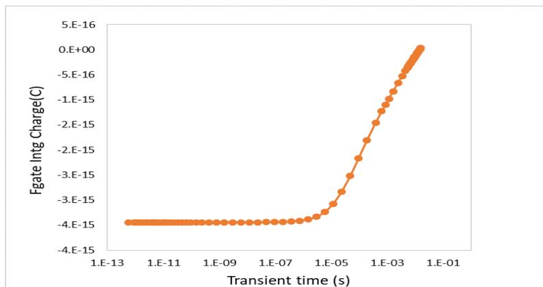
Fig. 12. Floating gate charge in erasing
