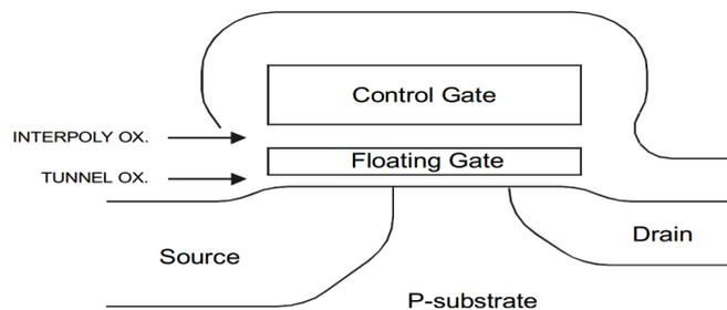
Fig. 1. Cross section schematic of a floating-gate device
