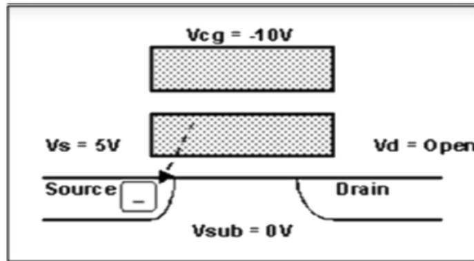
Fig. 4. Floating-gate erasing operation
