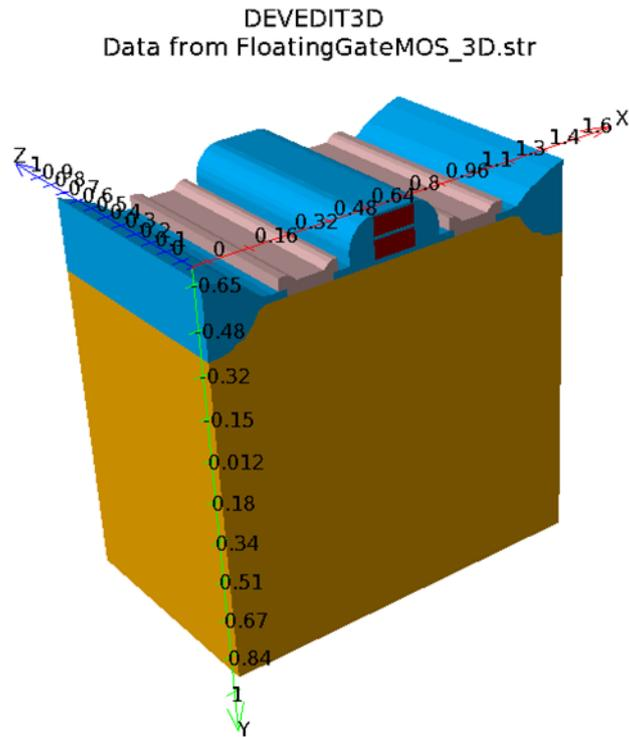
Fig. 8. The 2D structure of the floating-gate device
