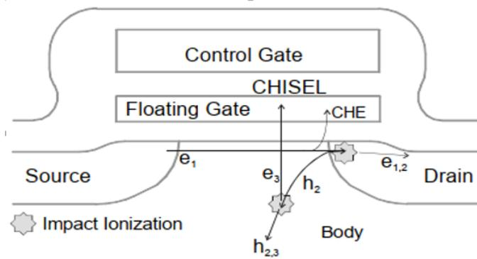
Fig. 3. Floating-gate programming operation
