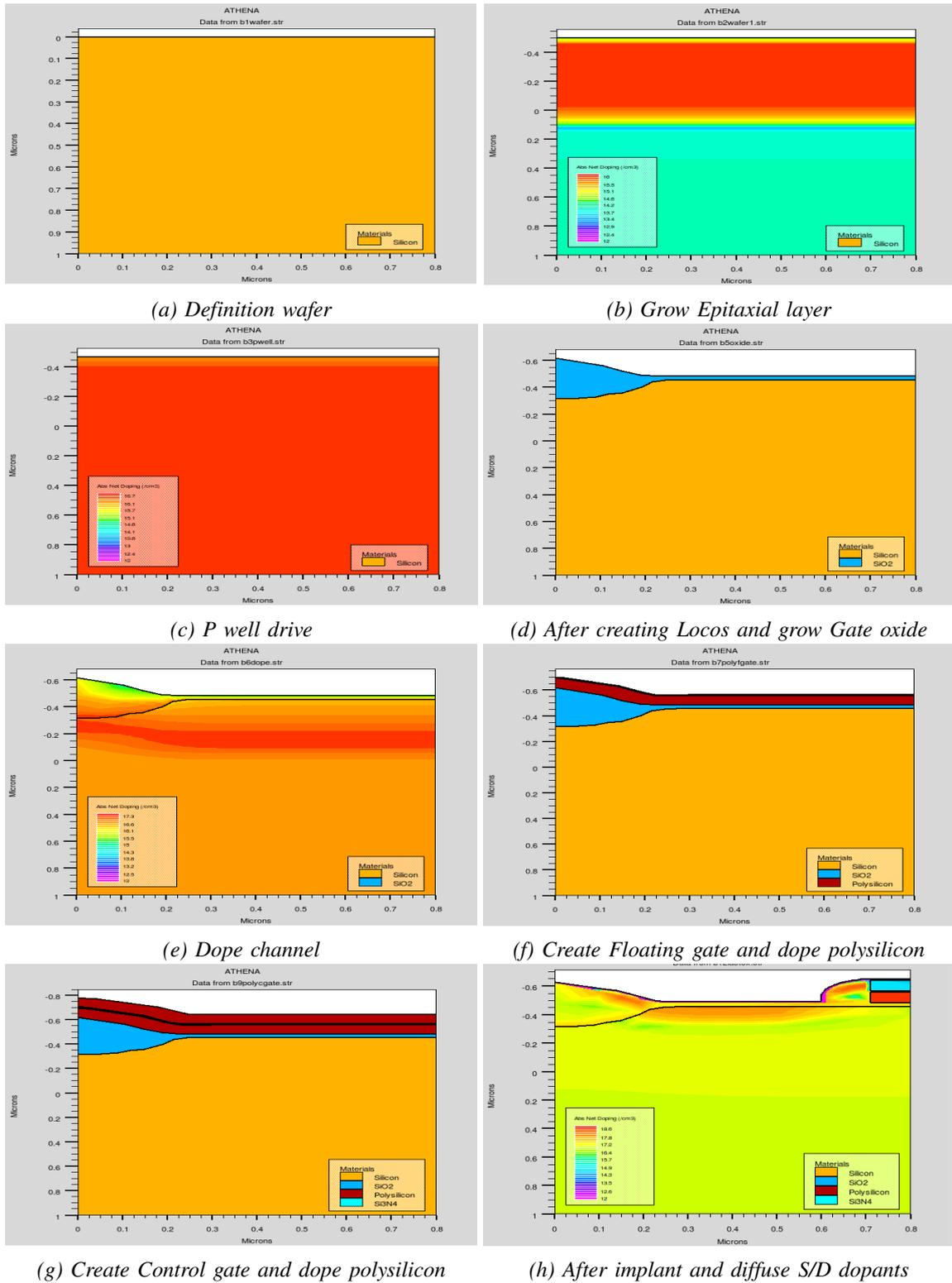
Fig. 6. The main process simulations with TCAD including in a) Definition wafer b) Grow Epitaxial layer c) P well drive d) After creating Locos and grow Gate oxide e) Dope channel f) Create Floating gate and dope polysilicon g) Create Control gate and dope polysilicon h) After implant and diffuse S/D dopants
