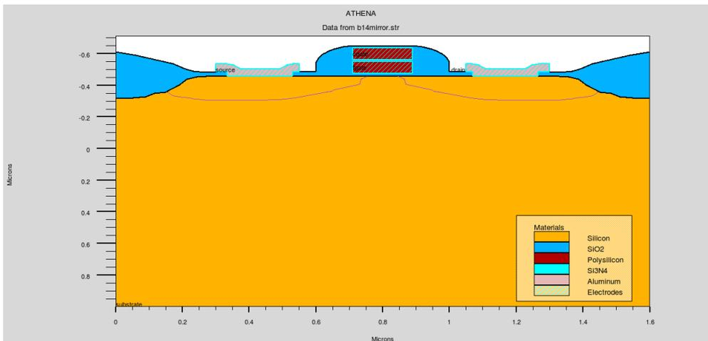
Fig. 7. The 2D structure of the floating-gate device
