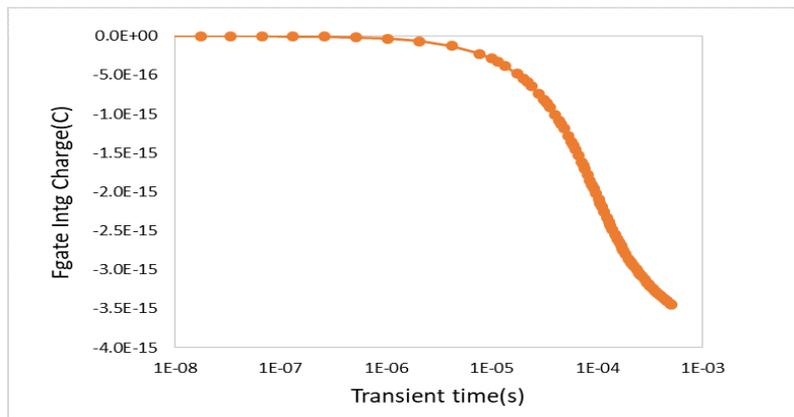
Fig. 10. Floating gate charge in programming
