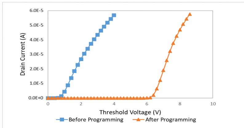
Fig. 11. Threshold voltage after programming
