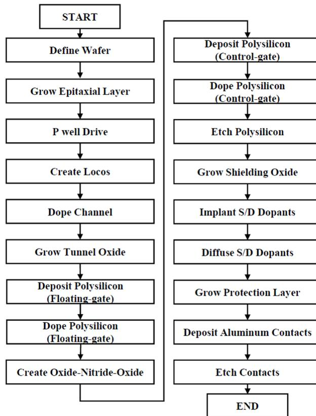
Fig. 5. Floating-gate device design flow chart
