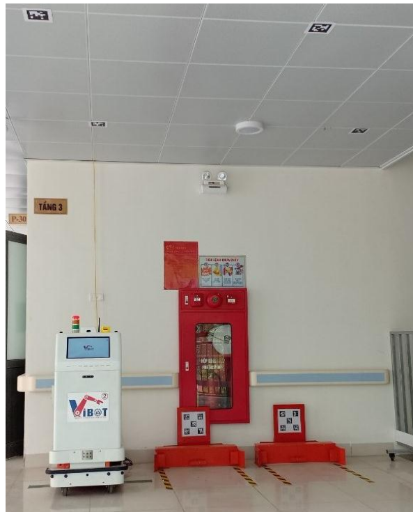
Fig. 3. AprilTags are mounted on the ceiling at Bac Giang general hospital.
