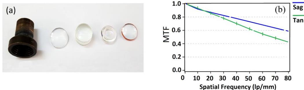
Fig. 4. (a) Objective's components; (b) Measured MTF of the objective.
