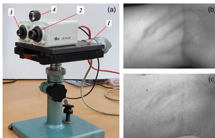
Fig. 5. (a) Experimental setup for capturing vein image: 1- Platform; 2- The camera is equipped with the near-infrared objective; 3- The camera is equipped with a typical objective; 4- Near-infrared LEDs. (b) and (c) Wrist images from cameras equipped with the near-infrared and typical objective, respectively.
