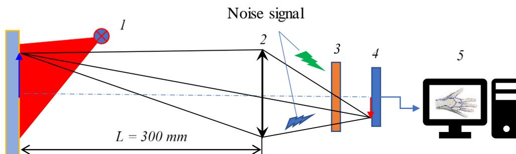
Fig. 1. Schematic diagram of a vein imaging system. 1- Near-infrared 850 nm LED; 2- Objective; 3- Optical filter; 4- Image sensor; 5- Image processing and display system.
