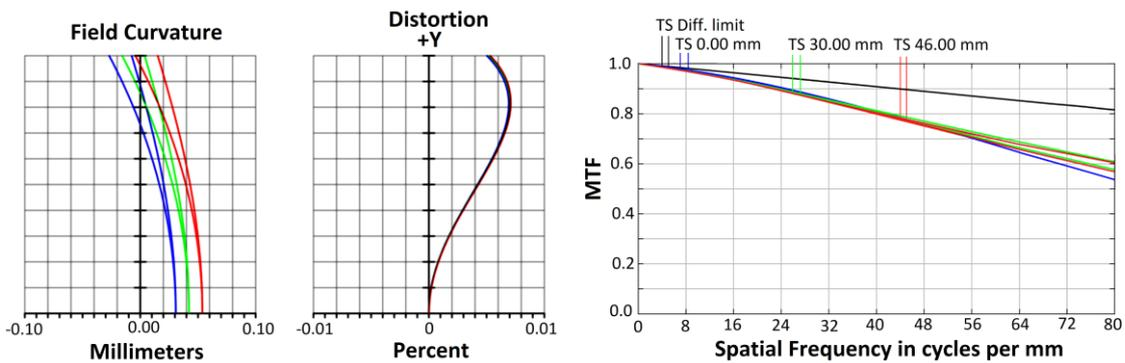
Fig. 3. (a) Field curvature and distortion of the objective. The wavelengths used are 850, 900, 950 nm; (b) MTF diagram of the objective.
