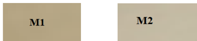
Fig. 2. Optical photos of the optical ceramic samples: the thickness of M1 (left) is 1.032 mm, the thickness of M2 (right) is 1.842 mm
