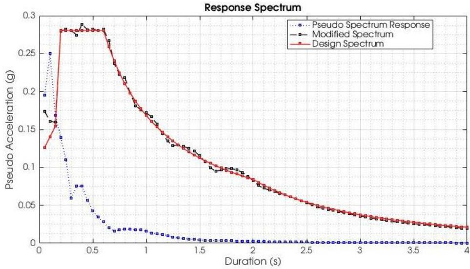
Figure 6. Results adjusting response spectrum for Dien Bien acceleration using PG01 program (BaDinh\_01C).
