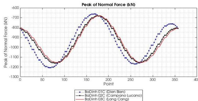
Figure 17. Survey results peak of normal force for 3 cases of load: BaDinh\_01C, BaDinh\_02C, BaDinh\_03C.
