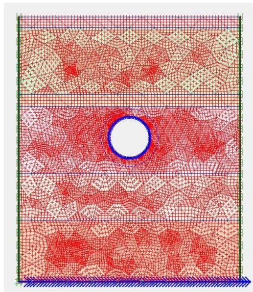
Figure 13. Element mesh of the model in Plaxis.
