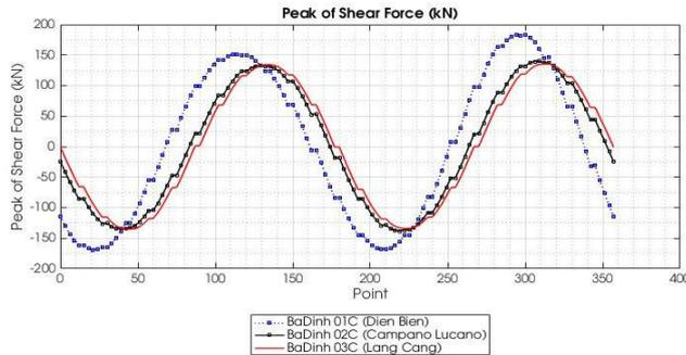
Figure 16. Survey results peak of shear force for 3 cases of load: BaDinh\_01C, BaDinh\_02C, BaDinh\_03C.
