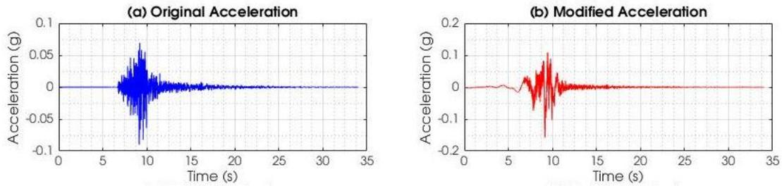
Figure 7. Original and modified acceleration with Dien Bien earthquake (BaDinh\_01C).
