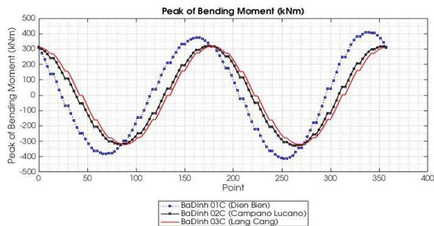
Figure 15. Survey results peak of bending moment for 3 load cases BaDinh\_01C, BaDinh\_02C, BaDinh\_03C.
