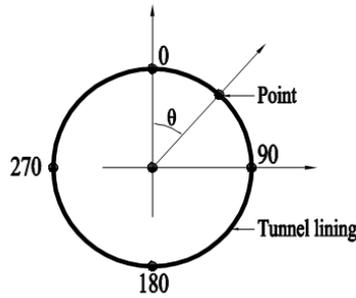
Figure 14. Conventional numbering points on the tunnel lining.
