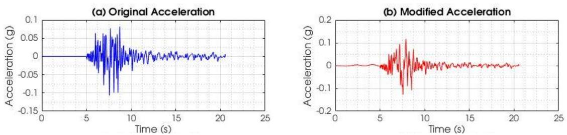
Figure 11. Original and modified acceleration with Lang Cang earthquake (BaDinh\_03C).
