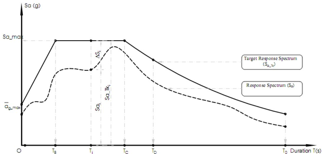
Figure 1. Response and target spectrum of acceleration.
