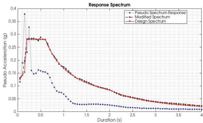
Figure 10. Results adjusting response spectrum for Lang Cang acceleration using PG01 program (BaDinh\_03C).
