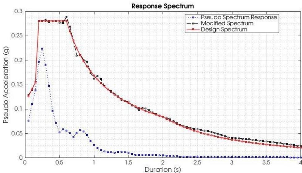
Figure 8. Results adjusting response spectrum for Campano Lucano acceleration using PG01 program (BaDinh\_02C).
