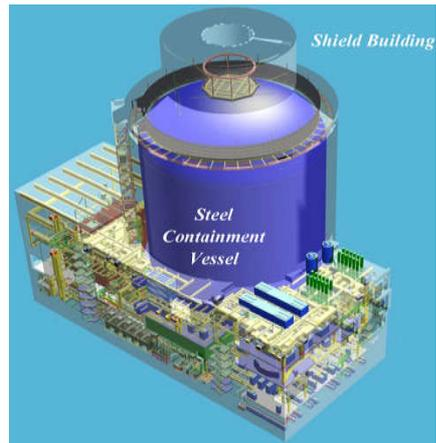
Figure 1. Main components of AP1000 nuclear island structure [4].
