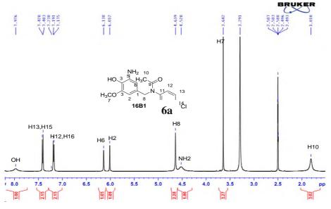
Fig.1. <sup>1</sup>H NMR spectrum of 6a
