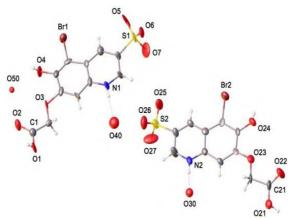
Fig.1. The spatial structure of QBr by single crystal X-ray diffraction measurements
