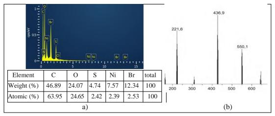
Fig.2. Result of EDX (a) and part of the +MS spectrum of NiQBr complex (b)
