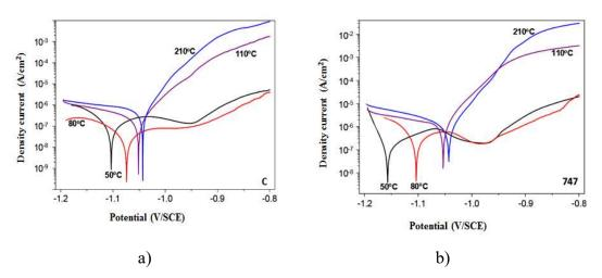
*Figure 3.* Polarization curves of conversion coatings produced in a - Cr (III)and b - conversion solution with various drying temperatures
