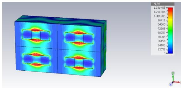
**Figure 4. Distribution of electric field at 758 GHz with the structure of 500 electrical conductivity doped silicon**
