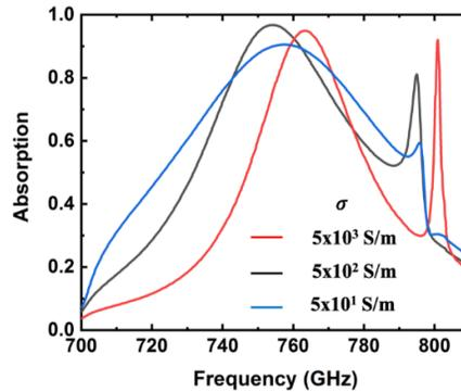
**Figure 3. Absorption of active region structures of TFTs using doped silicon with various electrical conductivities at the channel terminal**
