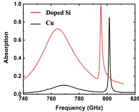
**Figure 2. Absorption of active region structures of TFTs using copper and doped silicon**
