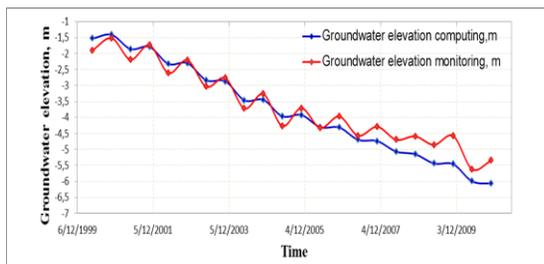
Figure 6. Computed and measured groundwater level at observation well Q40102t
