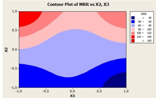
Figure 8. Two dimensional plot for effect of I and Ton on MRR
