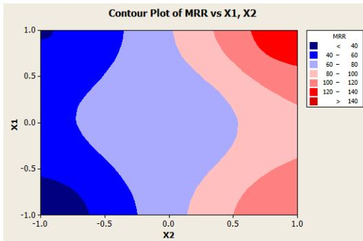
Figure 6. Two dimensional plot for effect of U and I on MRR
