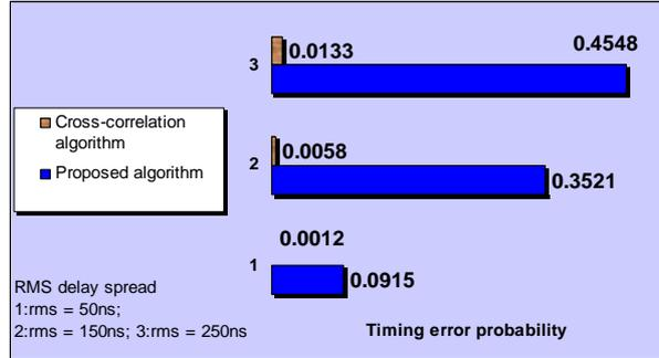
**Fig. 2:** Timing detection error probability in cross-correlation and proposed algorithms with  $2 \times 2$  antenna configurations
