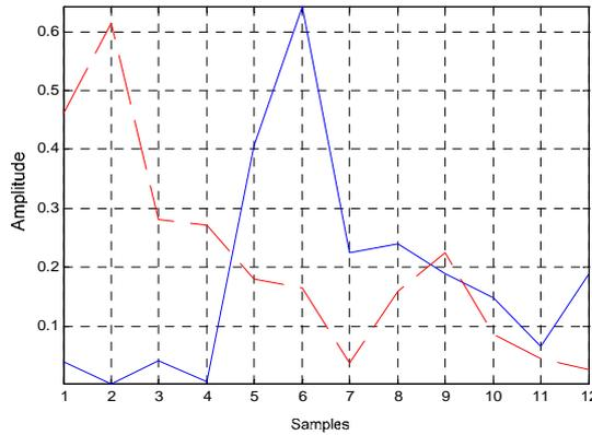
**Fig. 1:** 4-sample right shifted impulse response corresponding to 4-sample delayed detected timing
