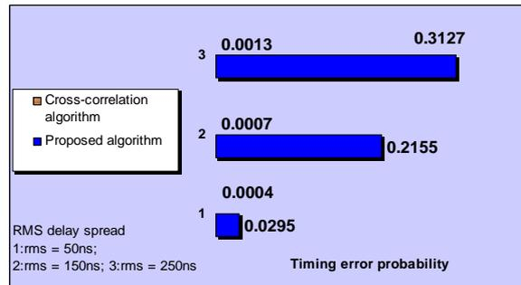
**Fig. 3:** Timing detection error probability in cross-correlation and proposed algorithms with  $2 \times 3$  antenna configurations
