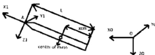
Figure 2 Axes of body and inertial frames.
