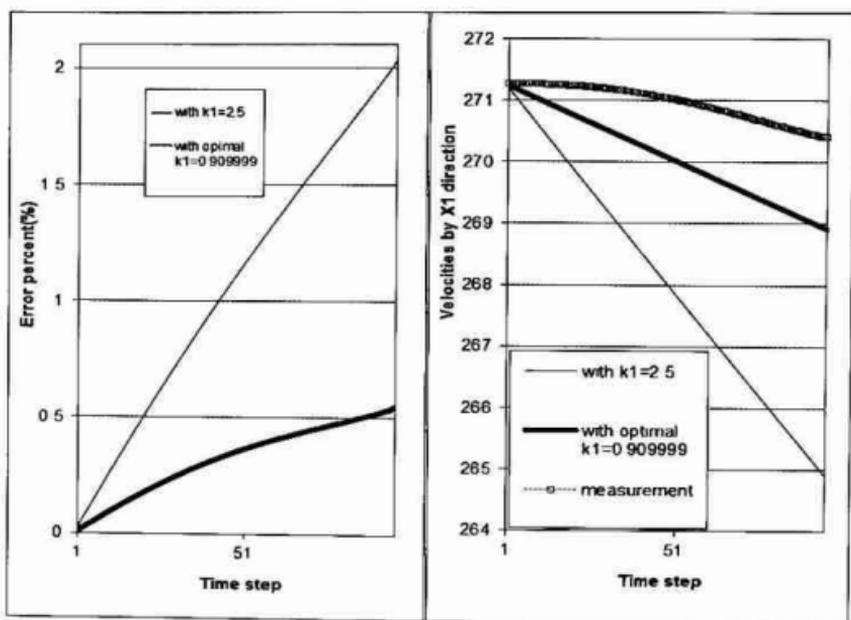
Figure 6 Percent error of velocities  $U$  by  $X_1$  direction with and without optimal correction of coefficient  $k_1$  comparing with measurement (left); Comparison of velocities  $U$  by  $X_1$  direction with or without correction and measurement.
