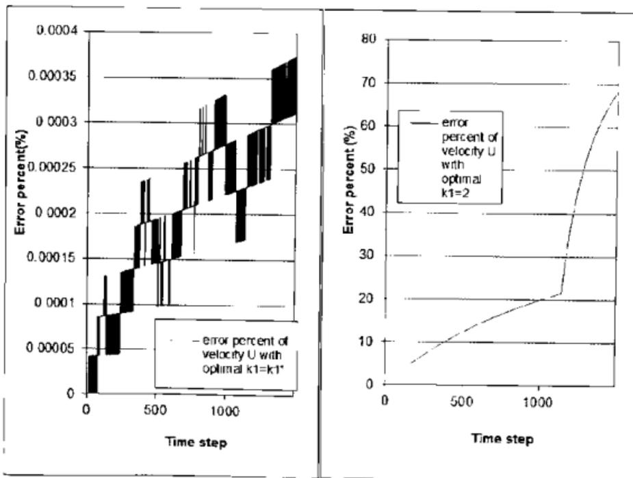
Figure 5. Percent error of velocity  $U(r)$  with optimal correction of coefficient  $k_1 = k_1^*$  (left), Percent error of velocity  $U(r)$  with coefficient  $k_1 = 2$  (Right)
