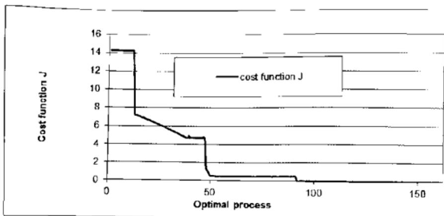
Figure 4. Cost function  $J$  in optimal process correcting  $k_1$ .
