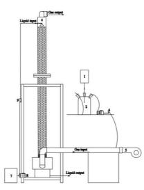
Fig. 2. Experimental set-up for chemical absorption of H<sub>2</sub>S in air: (1) sulfuric acid solution tank,
