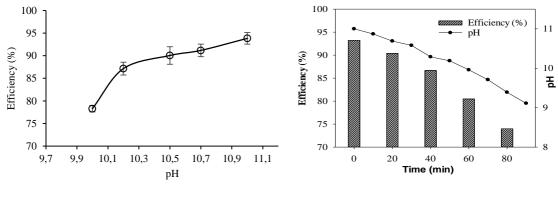
*Fig. 4.* Effect of initial pH on H<sub>2</sub>S removal efficiency (n = 3) (NaOH)
