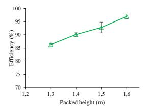
*Fig.* 7. Effect of packing height on the absorption efficiency (n = 6)
