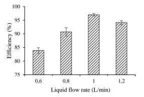
*Fig.* 6. The change of removal efficiency by liquid flow rate (n = 3)
