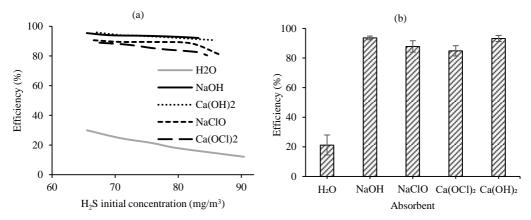
*Fig. 3.* H<sub>2</sub>S absorption efficiency of H<sub>2</sub>O, NaOH, Ca(OH)<sub>2</sub>, NaClO, and Ca(OCl)<sub>2</sub> (a) at different H<sub>2</sub>S initial concentrations and (b) at H<sub>2</sub>S initial concentration of 75 mg/m<sup>3</sup> (n = 5)
