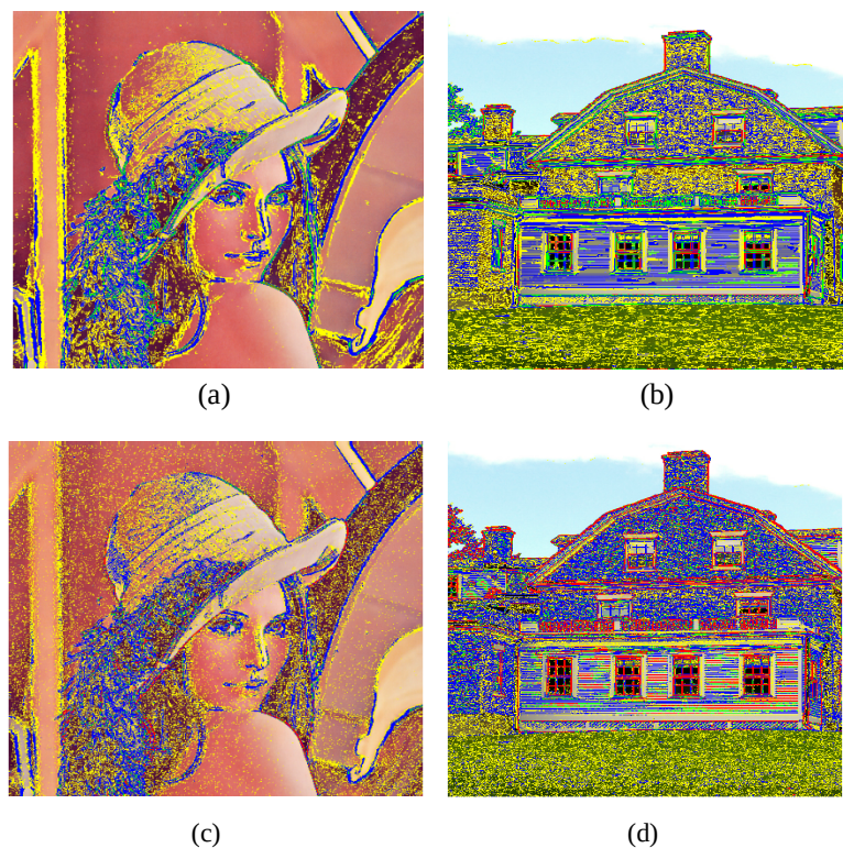
Figure 3. Texture map based on Sobel operator (a and b), and on pixel by pixel Beltrami method (c and d).
