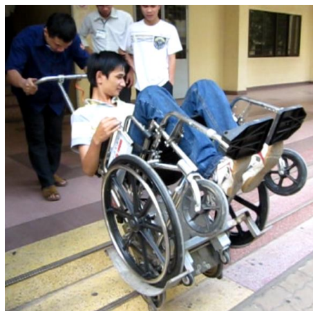
Figure 15. Machine climb down stair
