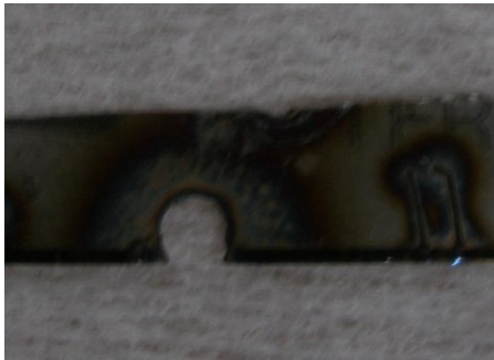
Figure 9. Photograph of cut-through hole on 100 \mu\text{m} steel plate (b)
